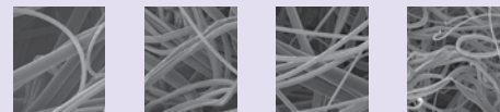
Outer pre-filter zone Inner pre-filter zone Final pre-filter zone Final filtration zone
